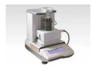
Automatic feature allow you analyze a dynamic hysteresis curve, complete with on-screen advancing, receding and zero depth of immersion results for contact angle or surface tension.
